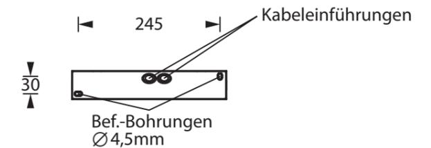
**Deckeneinbaumontage / recessed ceiling installation**
