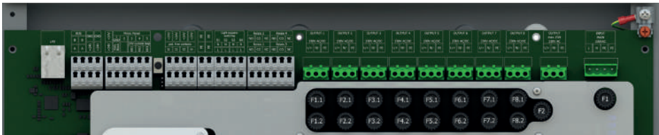
Fig. 18: Main board connection panel
