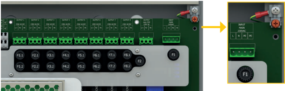
Fig. 19: Power supply connection
