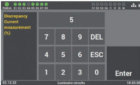
Fig. 91: "Threshold values" mask (electrical circuit monitoring)
