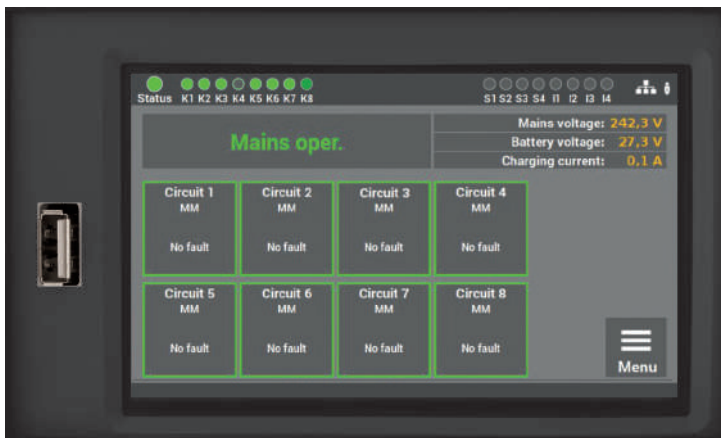
Fig. 31: USB connection at the display/front
