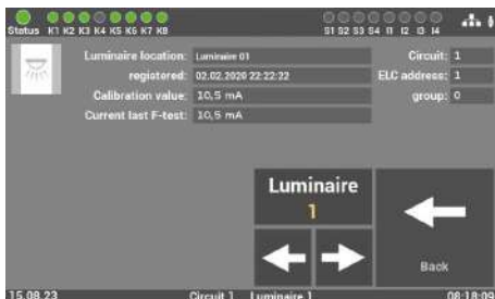
Fig. 54: Status of luminaire
